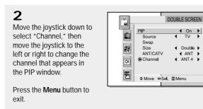
Note: The PIP channels are not available when RF is set to ANT-B. (The PIP channels link to ANT-A).
